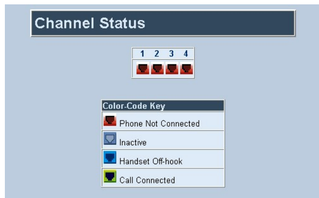
Figure 7-34: Channel Status Screen - FXO
