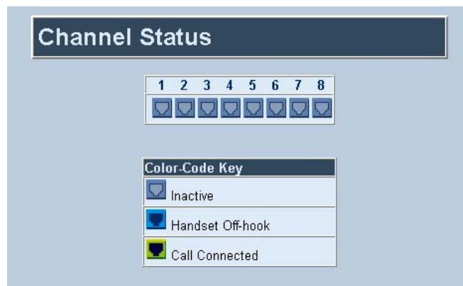
Figure 7-35: Channel Status Screen - FXS
